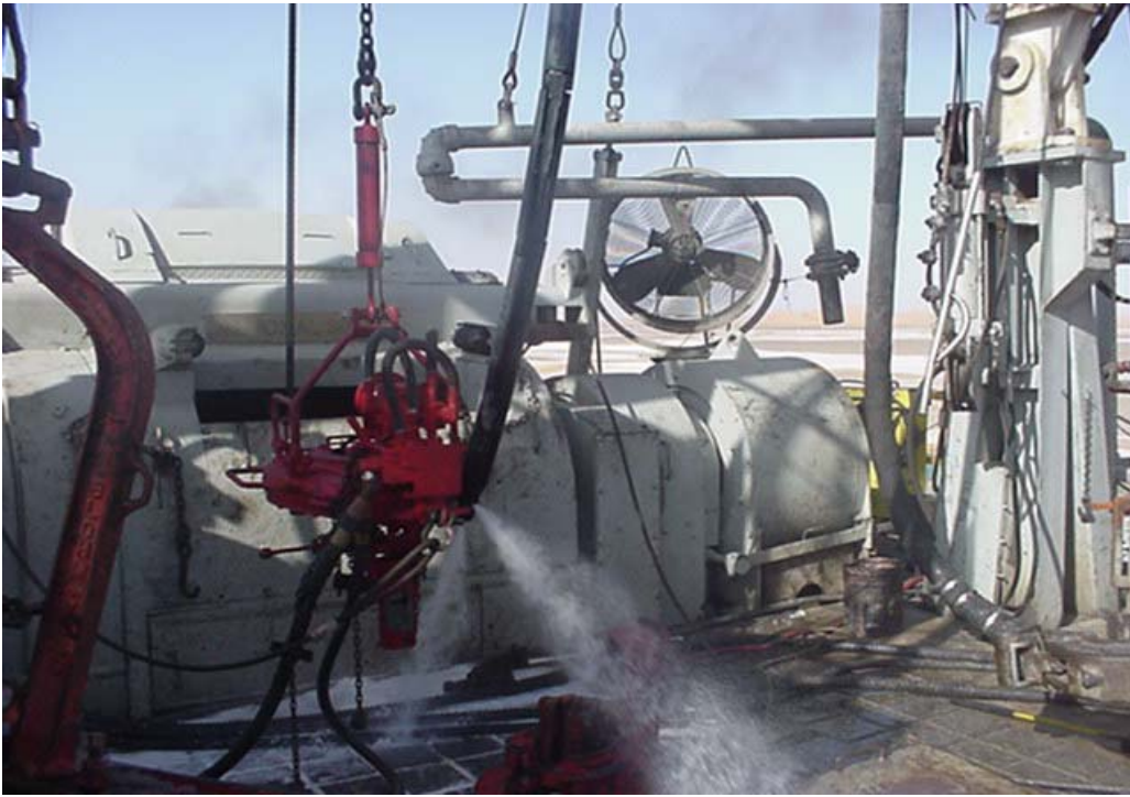
Fig-9 Surface test of the re-entry sub
